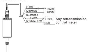
(D) 0~10V connect to Panel Meter series meter
